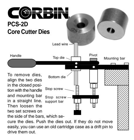
To install new dies, move the handle so about half the die hole is covered by the mounting bar (open position). Then, using the surface of the opposite bar as a stop, press the dies into place with the sharp edge of the die holes together, facing inward toward each other.
