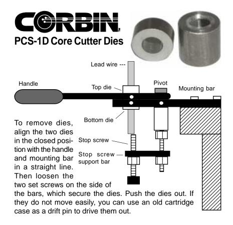
To install new dies, move the handle so about half the die hole is covered by the mounting bar (open position). Then, using the surface of the opposite bar as a stop, press the dies into place with the sharp edge of the die holes together, facing inward toward each other.
