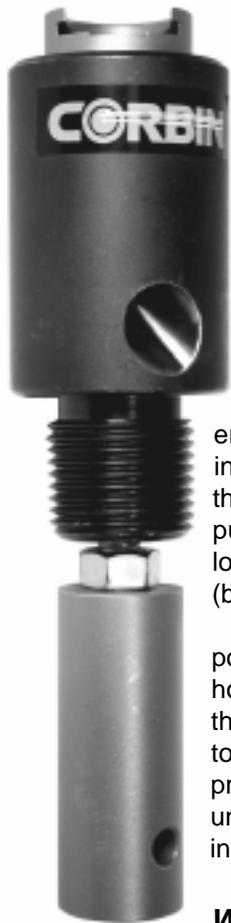
***A primer exhaust port*** in the side of the adapter unit allows spent primers to drop free of the press ram. Stretching the split end of a piece of clear vinyl tubing (3/4 inch or larger) around the adapter will allow the spent primers to drop into the tubing and roll down it, into a waiting container.
